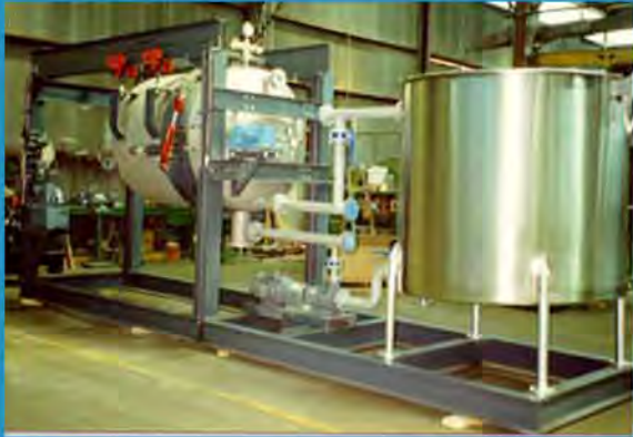
MCRO with vibrator and quick opening closure for dry cake discharge.
