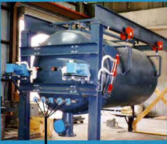
MCRO with vibrator and quick opening closure for dry cake discharge.
